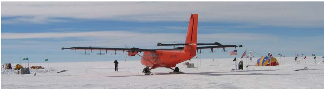
The BAS survey aircraft at PNE camp. Note the mag pods on the wingtips and the antennae array beneath the wings.
