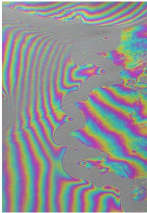
Example: RADARSAT-2 double difference interferogram showing a typical fringe pattern used to extract the GL. (Siple Coast)
