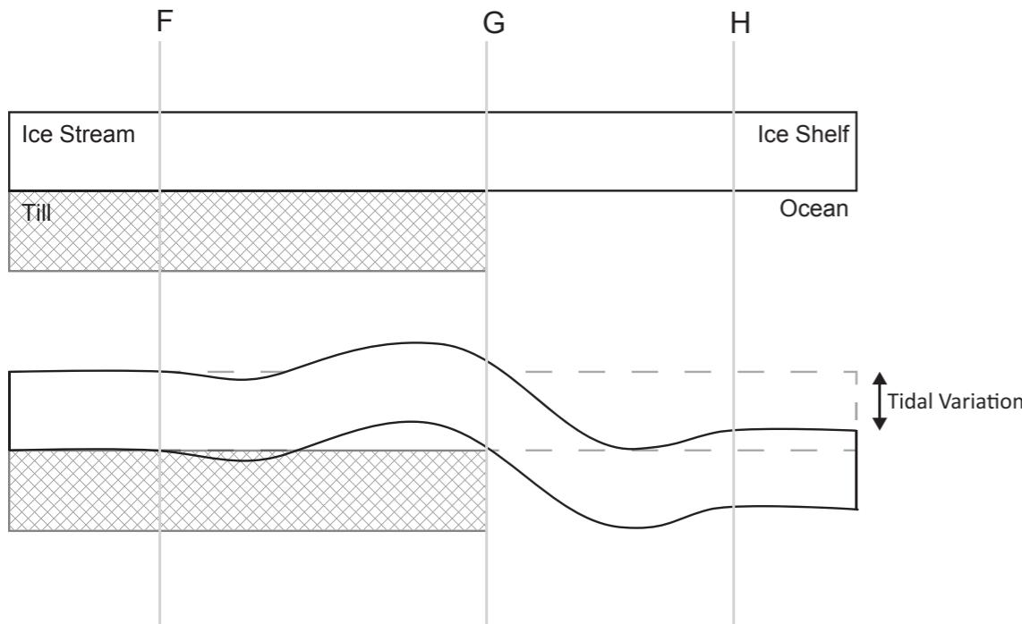
$$\frac{d^2}{dx^2} \left( D \frac{d^2 w}{dx^2} \right) = q - kw$$
