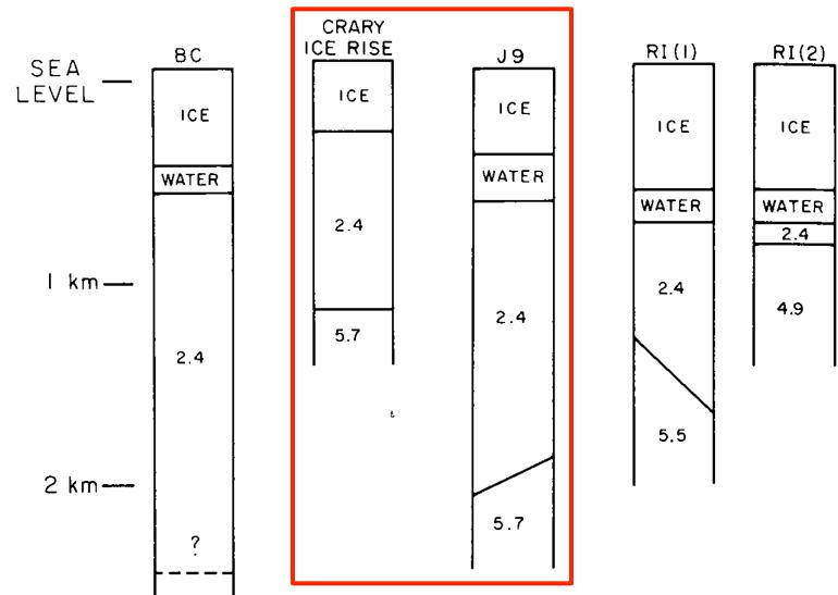
Figure 140.5. Seismic sections at station BC, Crary Ice Rise, station J9, and station RI; RI(1) is the preferred interpretation and RI(2) is an alternate interpretation. Numbers are seismic velocities in km/sec.
