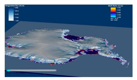
The figure shows the BISICLES-computed vertically-integrated ice velocity field about 1 month into a 20-year coupled Antarctic run, with the Filchner-Ronne ice shelf in the foreground. Grounding lines are shown in magenta. Subshelf melt rates are painted onto the ice shelves.
