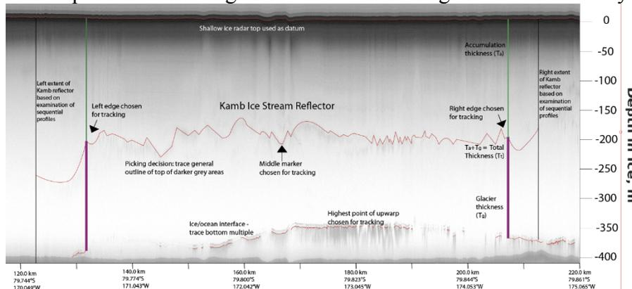
Annotated L660 radar-gram for Kamb Glacier, illustrating measurement method.
